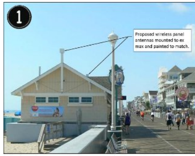
1. Custom wireless panel antennas mounted to match the building
