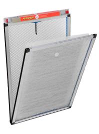
The Clean Air Defense System AirRanger™ whole house polarized-media electronic air cleaner installs directly into the 1" filter rack(s) in the existing heating and cooling system. Its electronically enhanced media combines elements of both electronic and media air cleaners. Particles are electrically charged (polarized) and then collected in the high efficiency media. Polarized sub-micron particles join with other particles and are collected on subsequent passes.
